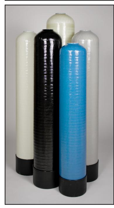
Clack Mineral Tanks are made of high density polyethylene (HDPE) plastic liner with composite fiberglass filament winding over the liner. Clack's design provides a continuous seamless inner liner with a glass filled polypropylene inlet for higher strength and pressure capabilities. Residential and commercial pressure tanks are available from 8" to 24" diameters.
